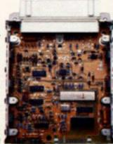
Control systems available in any production vehicle today. It continuously monitors all vital engine functions, and adjusts engine operation accordingly to maintain peak performance. EEC-IV also is programmed to compensate for changes that take place in a vehicle as it accumulates mileage and parts begin to wear.
