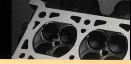
The SVT Cobra cylinder heads have two intake and two exhaust valves in each combustion chamber. The intake valves measure 37mm and the exhaust valves are 30mm in diameter.
