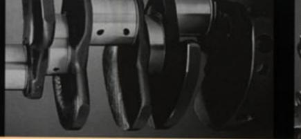
The forged-steel crankshaft is manufactured by Krupp Gerlach-Werke in the United States. Counterweights, placed opposite every throw of the crankshaft, contribute to the SVT COBRA engine's exceptionally smooth revving characteristics from idle to redline.
