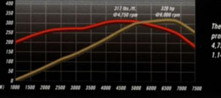
The SVT Cobra is free-revving from idle to its 6,800-rpm redline. It produces 320 horsepower at 6,000 rpm, and 317 lb.-ft. of torque at 4,750 rpm. The SVT Cobra V8 develops 69.55 horsepower per liter, or 1.14 horsepower per cubic inch.
