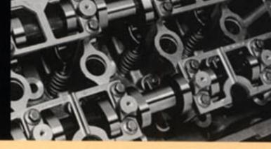
The camshafts run in line-bored journals and are secured from above with aluminum girdles. Roller-finger cam followers incorporate hydraulic valve-lash adjusters.
