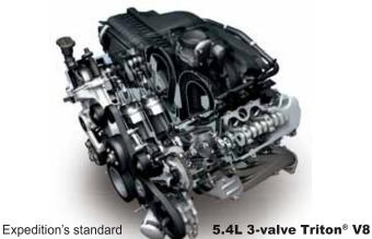
engine and automatic transmission are teamed with an Electronic Throttle Control system that responds more accurately to acceleration demands than a mechanical throttle cable, providing intuitive speed control, plus improved performance and fuel economy.
