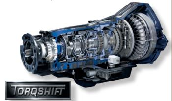
**TorqShift® 5-Speed Automatic** Its selectable Tow/Haul Mode is a true leap forward in towing performance. A sophisticated electronic control module adjusts operation to meet towing and hauling demands. The Tow/Haul Mode helps reduce gear hunting, improves power delivery, and even uses engine braking to help control vehicle speed when descending hills.
