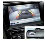
For visual assistance, a new Rear View Camera is available as part of the Driver's Vision Package and the Electronics Package. It puts a full-color image in the rearview mirror (on models without Navigation), or on the 8" screen of the available Navigation System. The available Reverse Sensing System sounds a warning to alert you of certain objects behind the vehicle as you slowly back up.
