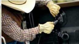
Makes connecting easy. Plug in your trailer wiring while standing upright with our class-exclusive in-bed 7-pin connector, part of the 5th-Wheel/Gooseneck Trailer Tow Prep Package!
