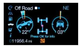
**Tracks the action.** You can monitor pitch angle, bank angle and wheel direction with our class-exclusive off-road display in the LCD productivity screen.2
