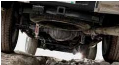
Maximizes your grip. Our electronic-locking rear differential<sup>2</sup> uses a true mechanical dog-clutch mechanism to lock the rear axle shafts together so they turn at the same speed.
