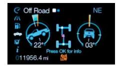
**Tracks the action.** You can monitor pitch angle, bank angle and wheel direction with our class-exclusive off-road display in the LCD productivity screen?
