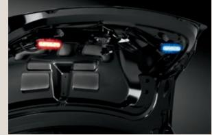
**Police trunk lights.** Includes (2) backlit flashing, linear high-intensity LED lights (driver side red; passenger side blue) – mounted on the inside of the trunk decklid. Lights activate when trunk is open.
