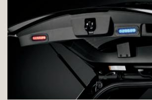
**Police liftgate lights.** Features (2) backlit flashing, linear high-intensity LED lights (driver side red; passenger side blue) – mounted inside the liftgate lip. Lights activate when liftgate is open.
