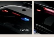
Police rear lighting. Includes (2) backlit flashing. linear high-intensity LED lights with surround cover (driver side red; passenger side blue). Sedan lights are mounted on the inside of the back window and Utility lights are mounted on the inside of the liftgate glass.
