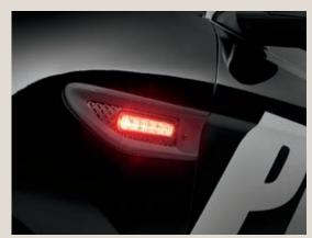
**Police side lamps.** Fender side markers feature backlit flashing, linear high-intensity LED lamps.
