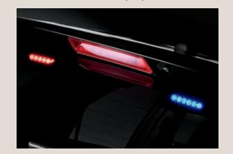
Police liftgate-glass lights. Includes (2) backlit flashing, linear high-intensity LED lights with surround cover (driver side red; passenger side blue) – mounted inside the liftgate glass.
