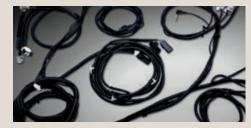
Wiring harness (Sedan). Includes (2) light connectors that support up to (3) LED lights each (engine compartment); (1) grille LED light connector that supports (2) LED lights; (2) 50-amp battery ground circuits in power distribution junction block (in-trunk); (1) 10-amp siren/speaker circuit (engine to trunk); trunk circulation fan; trunk electronics tray (4 sq. ft.); and pre-wiring for grille LEDs and siren/speaker.
