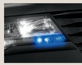
**Forward indicator pocket warning lamps.** Custom-designed, multifunctional Park/Turn/Warn (PTW) LED assemblies integrated into the headlamp system.
