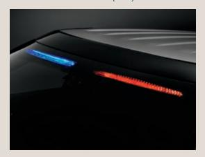
**Front interior visor light bar.** Includes (2) backlit flashing, linear high-intensity LED lights (driver side red; passenger side blue) – mounted inside the windshield glass. Lights can be programmed for tricolor (red, white, blue) patterns.
