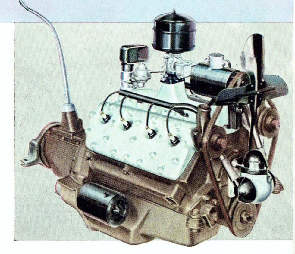
to own and drive. One is the tough, wearresisting cast-steel crankshaft. Another is directed-flow crankcase ventilation which gives to this enduring engine even longer life.
