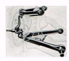
Ford's revolutionary new Ball-Joint Front Suspension is the finest available today. It provides a much smoother, quieter ride, cuts down on required steering effort, and retains more precise wheel alignment. Fragile merchandise rides gently. Here is a longer-lived suspension system that reduces maintenance, with only four lubrication points instead of customary sixteen.
