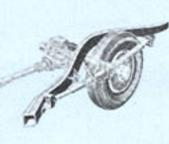
Heavy duty rear suspension . . Has extra-capacity spring leaves and heavy duty rear shock absorbers for handling big passenger loads with ease and comfort.
