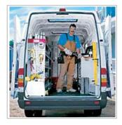
doors that open a full 270 degrees (the widest-opening doors in its class) on 140-inch and 158-inch wheelbase models—and stay open with magnets mounted to the exterior panels.
