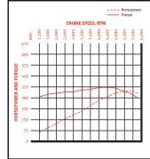
345\* horsepower @ 5,650 rpm 375 lb-ft of torque @ 4,200 rpm \*330 horsepower @ 4,800 rpm on 3500 models.
