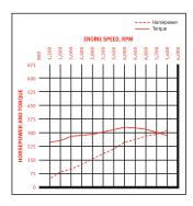
310 horsepower @ 5,650 rpm 330 lb-ft of torque @ 3,950 rpm
