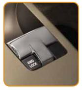
Compass's electronic coupling modulates when turning on a dry road in 4WD LOCK mode to help prevent noise.
