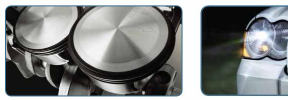
When the MDS feature on the 5.7L HEMI<sup>®</sup> V8 kicks in at cruising speeds, four of the engine's eight cylinders deactivate to provide fuel savings,<sup>(1)</sup> without giving up any power when you need it. New High Intensity Discharge (HID) headlamps have an auto-leveling feature that keeps them level, regardless of what you're carrying. Standard on Overland.
