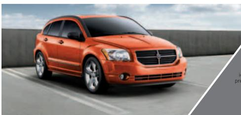
**RUSH.** Bright bodyside molding and exhaust tip. 2.4-liter DOHC 16V I-4 172-hp engine with dual VVT and five-speed manual transmission. Sport-suspension tuning. Sport Appearance Group with premium cloth seats with colored inserts, color-keyed instrument panel and shift console trim. Add ons: Leather Interior Group. Media Center 730N AM/FM/CD/DVD<sup>[2]</sup> radio with GPS Navigation and SIRIUS Satellite Radio (1-year subscription included). Security Group.
