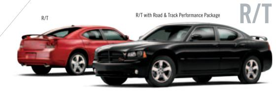
Includes the 5.7-liter Variable Valve Timing (VVT) HEMI V8 with MDS engine, 5-speed AutoStick® transmission, ABS, ESC with all-speed traction control, power driver and passenger heated leather-trimmed seats, leather-trimmed steering wheel with audio controls and shift knob, power adjustable pedals, vehicle information center, and 18-inch aluminum wheels and a rear spoiler.
