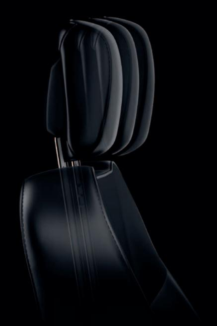
ACTIVE FRONT HEAD RESTRAINTS. (9) These help to reduce injury in a rear collision by minimizing the space between the head restraint and the occupant's head.
