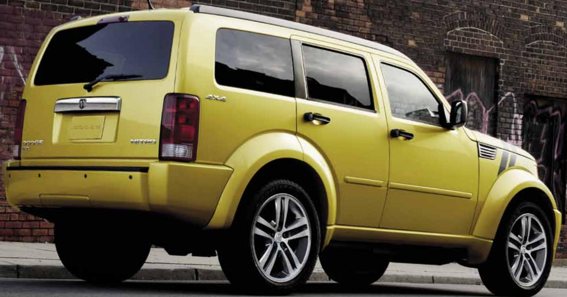
**NITRO PERFORMANCE.** Attitude without fortitude is meaningless, which is why Nitro Heat 4.0, Nitro Detonator and Nitro Shock are powered by a standard 4.0-liter V6 engine. Eager to unleash 260 horsepower and 265 lb-ft of torque, it's bolstered by a refined five-speed automatic transmission. A robust performance-tuned suspension helps to provide precise road handling. On 4x4 models, a part-time transfer case system gives you the ability to change from two-wheel to four-wheel drive on the fly.
