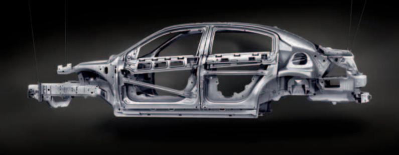
Specifically designed front and rear crumple zones help absorb energy and redirect it away from passengers, helping to reduce the risk of injury in the event of a collision.
