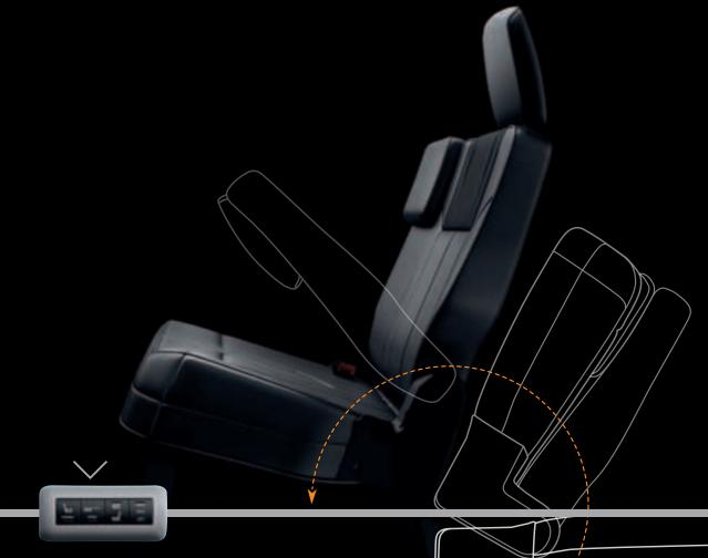
EXCLUSIVE ONE-TOUCH POWER-FOLDING THIRD-ROW SEATS. With the touch of a button the available class-exclusive one-touch powerfolding third-row 60/40 split-bench seat<sup>(1)</sup> folds directly into the floor. This feature also includes obstacle detection<sup>(2)</sup> to automatically pause if something is detected within the seat's path of motion.
