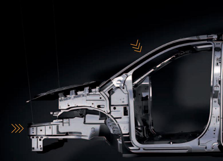
STRATEGICALLY PLACED HIGH-STRENGTH STEEL. The Town & Country architecture includes dual phase, high-strength and hot-stamped steel, resulting in a strong safety cage that contributes to overall vehicle-impact performance.
