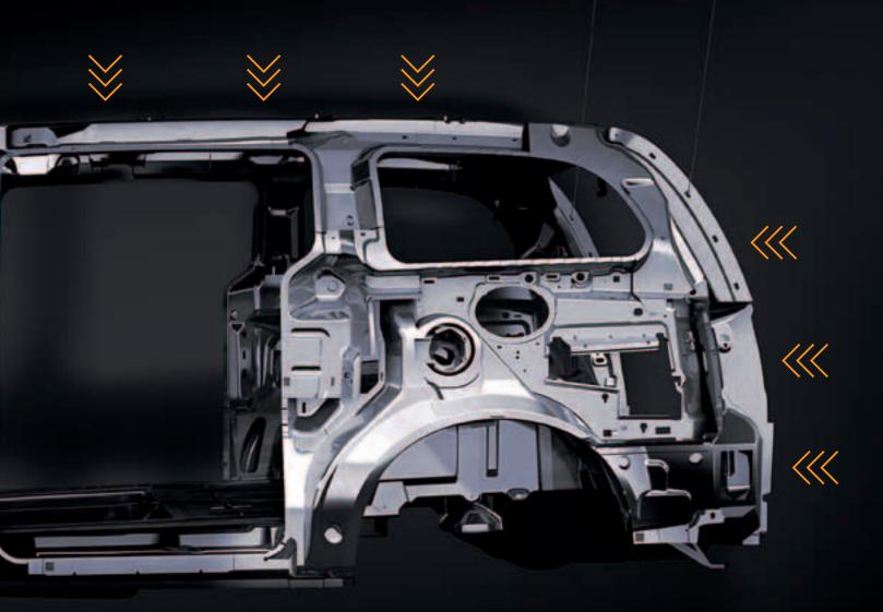
CRUMPLE ZONES. In the event of an impact, specifically designed front and rear crush zones absorb energy and redirect it away from passengers, helping to reduce the risk of injury.
