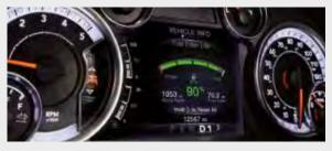
**NEW INSTRUMENTATION RUNS RINGS AROUND CONVENTION.** Select trim levels offer high-end electronics with a degree of sophistication never seen in Ram trucks. Assets include an available all-new six-ring instrument cluster with a 7-inch, fullcolor Multi-View Display with dozens of visual cues (telltales) for real-time information on truck functions, communications, and the radio. It's all operated through steering wheel-mounted cursors for instant menu access.
