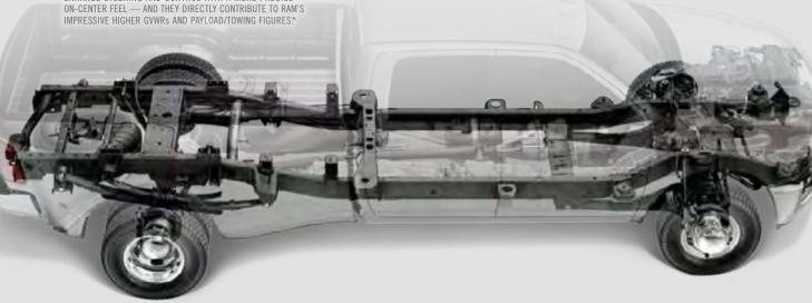
+ NEW 18- AND 20-INCH<sup>†</sup> WHEELS. AVAILABLE FOR RAM 3500 SINGLE-REAR-WHEEL MODELS, THEY ADD AUTHORITY TO THE NEW SCULPTED, FLOWING AERODYNAMIC EXTERIOR TOUCHES. + THE REVISED LADDER FRAME WITH EIGHT TOUGH CROSSMEMBERS AND WIDER RAILS ON NEW RAM 3500 LETS YOU TACKLE THE MOST CHALLENGING PAYLOADS WITH ASSURED CAPABILITY AND UNQUESTIONED STRENGTH.
