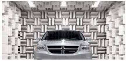
ANECHOIC CHAMBER — NOISE, VIBRATION AND HARSHNESS (NVH) TESTING
