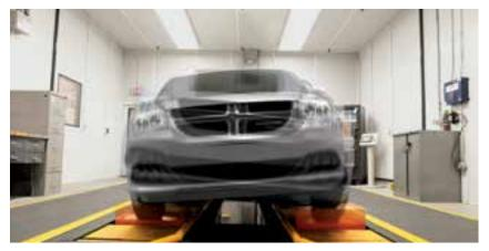
FOUR-POST SHAKER — SUSPENSION TESTING
