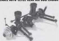
THE NEW AVAILABLE AUTO-LEVEL REAR AIR SUSPENSION SYSTEM\* FOR RAM 2500 is based on the available Active-Level™ Four-Corner Air Suspension System introduced by Ram I500, here in an operator-selectable two-mode configuration to accommodate the higher GCWRs of the weight class.
