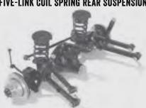
IT'S THE FIRST-OF-ITS-KIND REAR SUSPENSION FOR A HEAVY-DUTY PICKUP and it's the standard for Ram 2500 models. The class-exclusive<sup>[I]</sup> five-link coil spring rear suspension features unique, multirate coil springs and heavy-duty fixed-displacement twin-tube shock absorbers; both are placed in a more outboard position that optimizes performance and minimizes noise/vibration. A huge II.5-inch solid rear axle rounds it out for exceptional handling, especially when carrying heavy loads.
