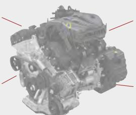
Torque is critical. The Pentastar V6 torque curve exceeds 90 percent of the peak value in the I,600–6,400 rpm range — ideal calibration to provide power along with smooth and responsive driving.
