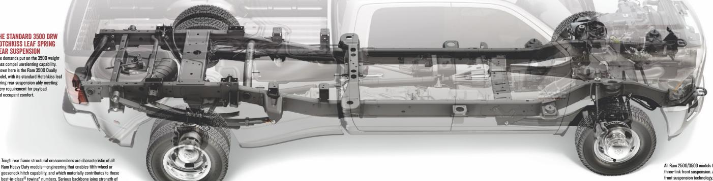
All Ram 2500/3500 models feature as standard equipment the unique three-link front suspension. As well as incorporating the three-link front suspension technology, we also integrated a large stabilizer bar to ensure the roll stiffness required by the high GVW ratings of Ram Heavy Duty. Those numbers are impressive, reaching up to 10,000 lb for Ram 2500 and up to 14,000 lb for Ram 3500 models.
