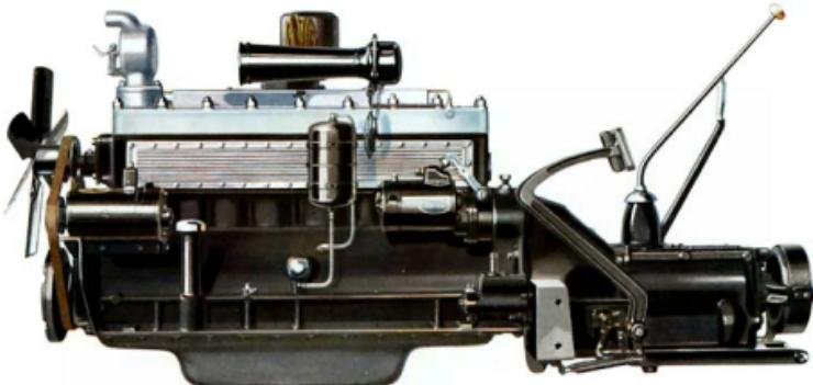
The engine of the Chrysler Imperial Eight—the outstanding triumph of the most progressive group of engineers in the industry, is an achievement in high powered smoothness such as eight cylinders have never been known to produce. It develops 125 horsepower at 3200 revolutions per minute.
