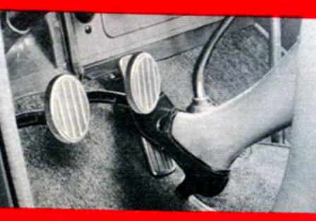
At or above 35 miles an hour, when the overdrive transmission is in operation, momentarily lift your foot from the accelerator pedal and the lower gear ratio goes into operation.
