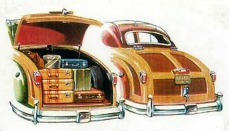
The rear deck is beautifully rounded to complement the long, flowing lines of the body. Deck-lid is counterbalanced and can be easily raised or lowered.
