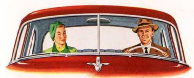
LIKE ALL PLYMOUTHS, this model has exceptional all-around vision. The front pillar posts are narrower, the rear-view mirror is wider, and the rear window is larger than in previous models.
