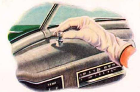
New Electric Windshield Wipers operate at a constant speed regardless of engine load or speed of the car. They do not slow up or stop when car is climbing a hill or accelerating. This is very important when passing another car in wet or stormy weather. Wiper blades clear almost three-quarters of the windshield area,
