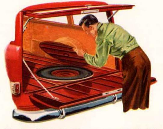
THE SPARE TIRE is out of the way, yet easy to get at, for it is housed in a well, under a flat cover which forms part of the floor. With the rear seat folded into the floor, there is 66¾" of unobstructed floor space from the back of the front seat to the tail gate; with the tail gate down, there is a total of 87¾" usable space.
