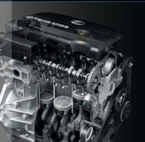
An advanced MZR 2.5-liter DOHC engine to deliver both spirited performance and an enviable 22 MPG city/28 MPG highway.\* The Mazda5's advanced Electrohydraulic Power Assist Steering utilizes hydraulic pressure from a pump driven by an electric motor that works independently of the car's engine, resulting in increased fuel economy, improved pin-point steering power and enhanced agility.
