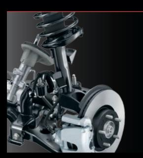
Standard lightweight aluminum alloy wheels help reduce unsprung weight, improving handling. 4-wheel independent suspension provides a smoother, more responsive ride, while 4-wheel anti-lock brakes maintain steering control during emergency situations.
