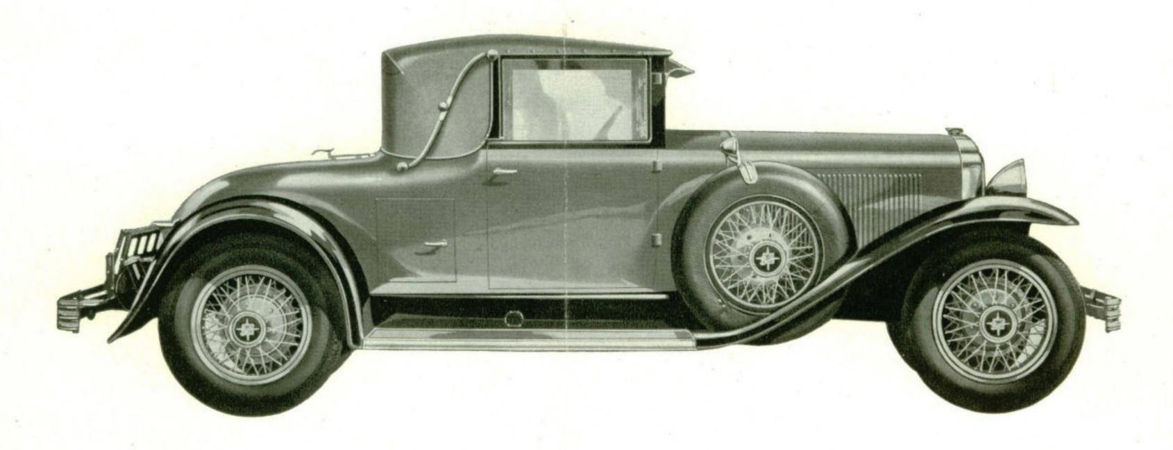
Four-Passenger Convertible Coupe (Series 129) A luxurious sport model providing a quickly-lowered top, entirely separate from the doors, so that side windows may be raised to windshield height with top down. The car closes tightly with top raised. Special features include commodious rumble seat with comfortable accommodations for two, and a side-opening compartment for golf equipment or other luggage.
