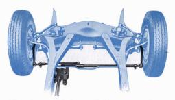
The steering assembly has been simplified for greater strength and easier maintenance. Steering is, if anything, lighter than in previous models, as a result of this new design.
