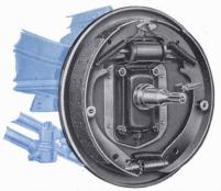
Buick's tiptoe hydraulic brakes are of the internalexpanding type, utilizing the motion of the car to supply brake effect, which naturally reduces needed effort at the foot pedal. In addition, wear on brake bands is more even than in brakes of other types.
