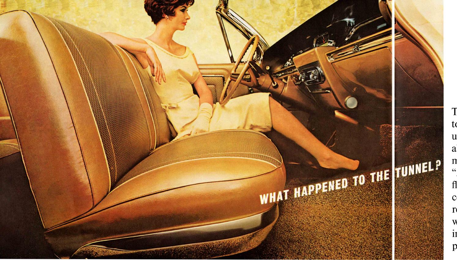
Time was when all automobile floors were flat. Then automobile bodies started to descend. The drive shaft (an indispensable item) had no place to go but up into the passenger compartment. Drive shaft tunnels reached truly formidable dimensions.
