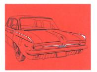
\*Rear Fender Peak Moulding and Rear Deck Applique (3) (4)
