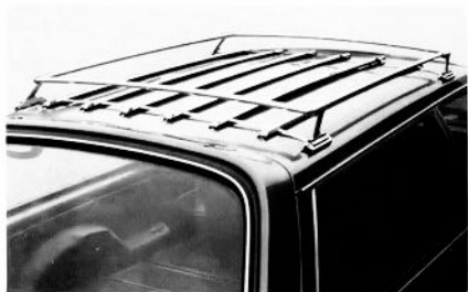
Hatchback Luggage Carrier (Code 524—UPC V55). Chrome and stainless steel. Permanently installed. Side rails for easy tie-down. Available. Aste, Aste SJ, Ventura, Ventura Custom and Ventura SJ. (Shown on Aste Safari) (F, D)
