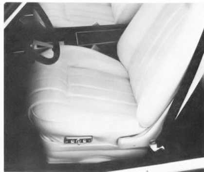
Six-way Power Bucket Seat, Left-hand Only (Code 561—UPC AC3). Raises, lowers, tilts forward or backward, or moves forward or backward. Available with bucket seats on LeMans Sport Coupe, Grand LeMans 2- and 4-door, Grand LeMans Safari, Grand Am and Grand Prix. (F)
