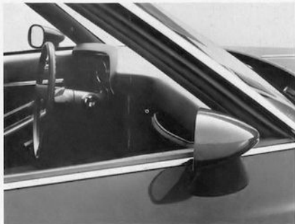
Remote Controlled Sports Mirrors (Code 424—UPC DF4). Body colored. Right- and left-hand. Available on all models except Astre and Firebird models. Standard with Grand Prix LJ Package with bucket seats only. Available on Grand LeMans, Grand Am and Grand Prix with console only. (F,D)
