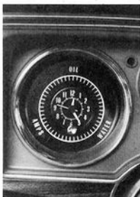
Electric Clock (Code 711—UPC U35). Illuminated dial, sweep second hand and automatic regulator. Standard on Astro S2, Astro SJ Safari, Grand LeMans, Grand LeMans Safari, Grand Am, Grand Ville Brougham, Grand Safari and Grand Prix. Available on all other models. Available on Catalina and Bonneville (Code 502—UPC U35). (F,D)
