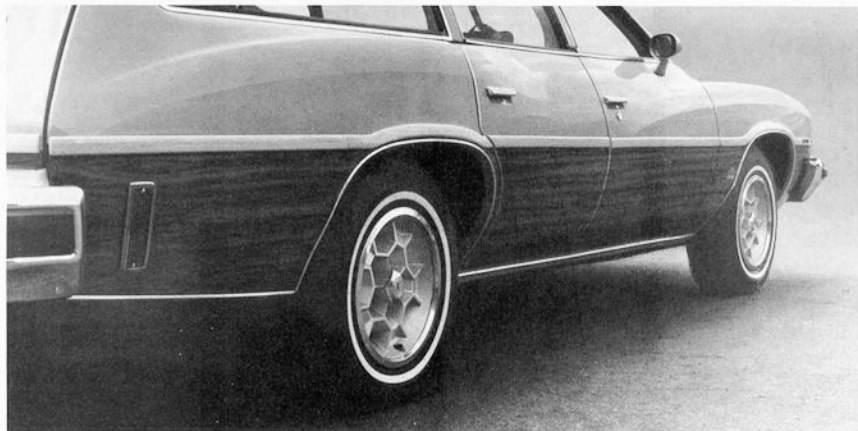
Woodgrain Appearance Siding (Code 512—UPC W61). Walnut woodgrain vinyl is translucent to allow body color to show through slightly. Available on Astre Safari, Astre SJ Safari, LeMans Safari, Grand LeMans Safari, Catalina Safari and Grand Safari. (F)
