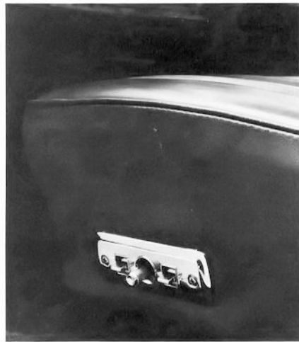
Six-way Power Full-width Seat (Code 561—UPC A42). Raises, lowers, tilts forward or backward, or moves forward or backward. Available on all models except Astre, Venture and Firebird models. When 60/40 seat is ordered on all models except Grand Am, driver's side can be powered (Code 561—UPC AG1), with manual passenger adjustment. Passenger side can also be powered (Code 562—UPC AG2). (F)
