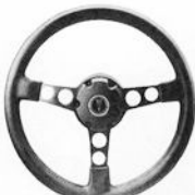
Formula Steering Wheel (Code 464-UPC N33). Black only. Available on Astre models. Available on Firebird, Firebird Esprit, Firebird Formula and standard on Firebird Trans Am with Firebird emblem replacing Pontiac crest. (F)
