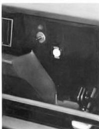
Deck Lid Release (Code 702—UPC AS0). Just press the button inside the glove compartment or console to unlock the trunk. Trunk also can be opened and closed in the conventional manner. Available on all models except wagons, Ventura and Astre models. (F,D) Dealer installed only on Firebird models.
