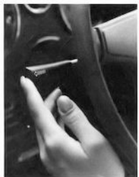
Cruise Control (Code 564—UPC K30). Attain desired speed, lightly touch the button in the end of the turn signal indicator, release accelerator pedal, and car will maintain that speed. Car can be accelerated, then will drop back to setting with release of accelerator. To disengage, simply touch the brake pedal. Available on all models with V-8 engines and Turbo Hydra-matic transmissions except Astre, Ventura and Firebird models. (F,D)
