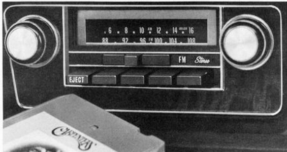
Stereo AM/FM Radio/Tape Player (Code 409—UPC UM2). Radio and tape player combine into a single unit with radio dial face functioning as the tape player door. (System has multiple speakers.) (F,D) FM radio plays in full stereophonic sound with stereo broadcasting. Also with AM Radio, only (Code 407—UPC UM1). Available on all models except Astre models and Firebird models. (F,D)
