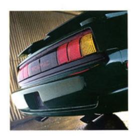
The new rear wing for the GTA is shaped like an inverted airfoil for enhanced effectiveness. The chrome tailpipes are fair warning of the potential rumbling in its 235 hp exhaust.
