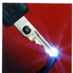
PASS-Key\* is the key to peace of mind for Firebird owners. The dark insert in the key shank is a specific resistor. Without its "code", special systems will prevent the car from starting.
