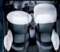
Dual front airbags<sup>2</sup> and front side airbags, both standard, protect the driver and front passenger.
