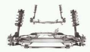
**Sport-tuned suspension system**. Standard equipment on the SC2, this system includes both front and rear stabilizer bars and stiffer springs that help provide a firm, solid ride while minimizing the transmission of road imperfections to the interior. The result is excellent control and a comfortable ride. The suspension system is a natural fit with Saturn's rigid spaceframe chassis.
