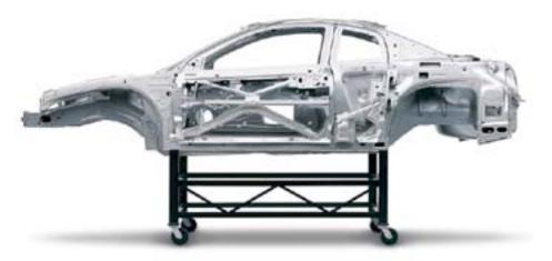
Steel spaceframe construction. Every three-door coupe is built on a strong, welded steel skeleton. Front and rear crumple zones are designed to help absorb energy instead of transmitting it all to the passengers. The doors are built with steel beams and cross bracing for side-impact protection. As if the intended safety benefits weren't enough, this construction also helps reduce the number of squeaks and rattles that can develop over time.
