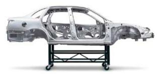
**L-Series modified spaceframe.** If automobile safety had a heart, this would certainly be it. A steel structure that encases the passenger compartment and is designed with front and rear crumple zones to help absorb the energy from a crash. There's also a great side benefit to the solid design—fewer squeaks and rattles down the road.
