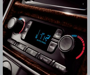
I. The automatic dual-zone climate control lets you dial in a difference of up to 25°F between driver and front passenger.
