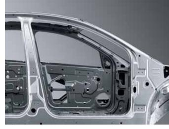
BUILDING CONFIDENCE. We gave the AURA a high-strength steel-reinforced safety cage as well as front and rear impact-absorbing crumple zones. Steel side-intrusion beams in the front doors provide front passengers with even more peace of mind.
