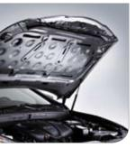
HOOD STRUCTURE Sonata was designed with hood-buckling creases to help protect you in an impact from any direction.
