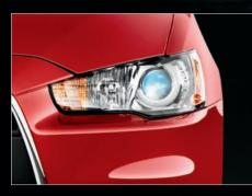
Available Auto On/Off Bi-Xenon HID Headlamps High-Intensity Discharge (HID) headlamps use xenon gas. They last longer and emit more light than halogen headlamps. Even better, the light quality of xenon gas more closely mimics that of the sun, making for better definition and less eye fatigue.
