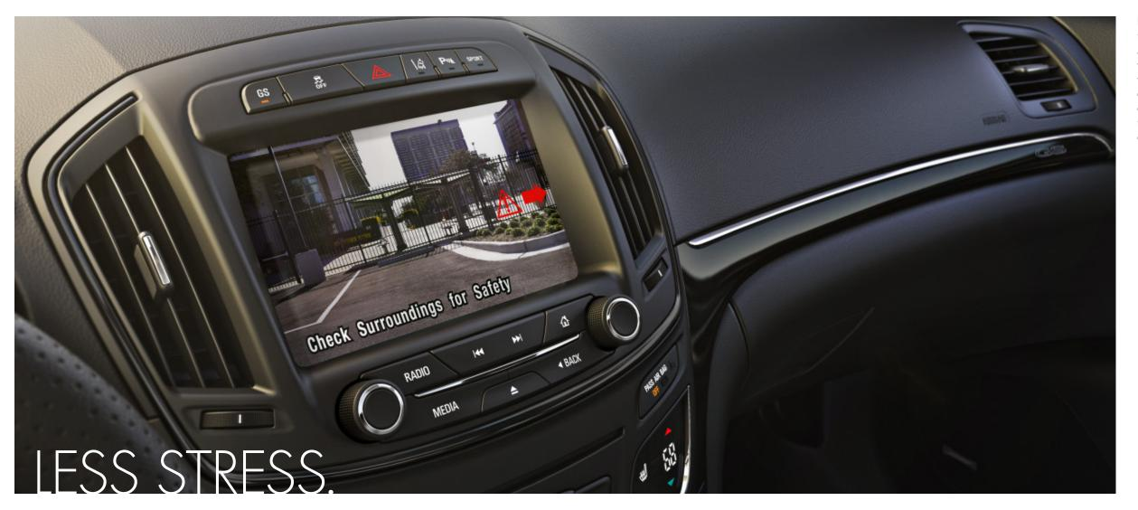
REAR CROSS TRAFFIC ALERT. Among the safety features that are offered on the new Regal is Rear Cross Traffic Alert. A camera in the rear captures a view behind the vehicle when backing up, while radar sensors detect vehicles approaching from the left or right. If the system detects a vehicle approaching within 65 feet in either direction, an alert sounds and warning indicators on the rear vision camera screen will alert the driver to help avoid backing into approaching traffic.
