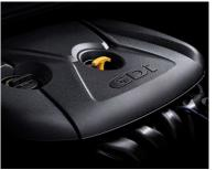
**ADVANCED ENGINE TECH** The Elantra's available 2.0-liter engine draws its responsive power from Gasoline Direct Injection (GDI) and Dual Continuously Variable Valve Timing. GDI atomizes fuel directly into each cylinder's combustion chamber for added power and greater fuel efficiency with cleaner emissions.
