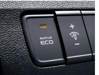
**ACTIVE ECO SYSTEM** At the press of a button on the dashboard, Elantra's Active ECO System modifies engine and automatic transmission controls to smooth out shift points and help boost fuel efficiency.<sup>3</sup> With prices at the pump being what they are, every extra drop counts.
