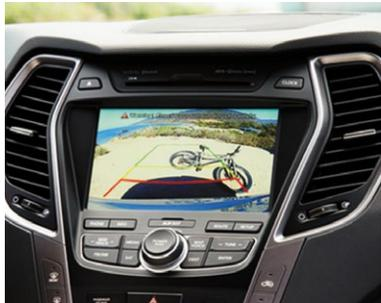
**REARVIEW CAMERA** Santa Fe's available 8-inch navigation and 4.3-inch touchscreen audio systems feature a rearview camera that displays views from behind the vehicle on a central in-dash screen. Guidelines on the screen help direct you through tricky turning maneuvers or into tight parking spaces when backing up your Santa Fe.
