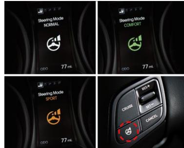
**SMARTER STEERING** Santa Fe Sport is the first CUV to feature Driver Selectable Steering Modes, which allow you to choose your preferred mode of power steering – Comfort, Normal or Sport – using a button on the steering wheel for a more customized feel behind the wheel.
