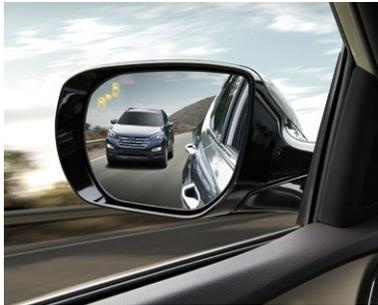
**VISIONARY TECH** For added help seeing what's around you, Santa Fe now offers two advanced technologies. A Rear Parking Assistance System helps you back into parking spaces, while Blind Spot Detection flashes an alert in the driver's side mirror whenever a vehicle enters the blind zones alongside your Santa Fe.
