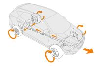
**ALL WHEEL GRIP** To help optimize traction when the going gets tricky, Tucson's available All Wheel Drive continuously varies the torque transfer between front and rear wheels automatically. Drivers can also select the 50/50 torque-split setting to balance power between front and rear wheels in snow or deep sand conditions.
