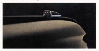
you, such as lamp monitors that tell you whether your headlights, rear lights and turn signals are functioning properly. Coupled with the lamp monitoring system is a warning light that lets you know when your windshield washer fluid is low.
